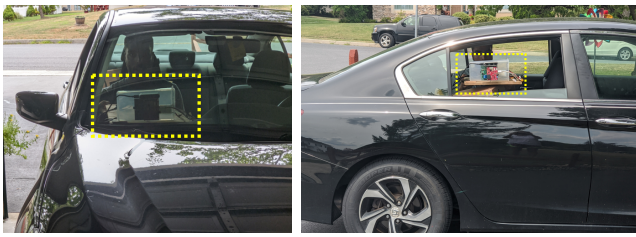
Fig. 10. The two ways in which the radar system was mounted in the moving vehicle for the scenes on the road. In both cases, there was a window in front of the system. For the data from the front facing radar, there are reflections caused by the front of the car, namely the hood and engine.
